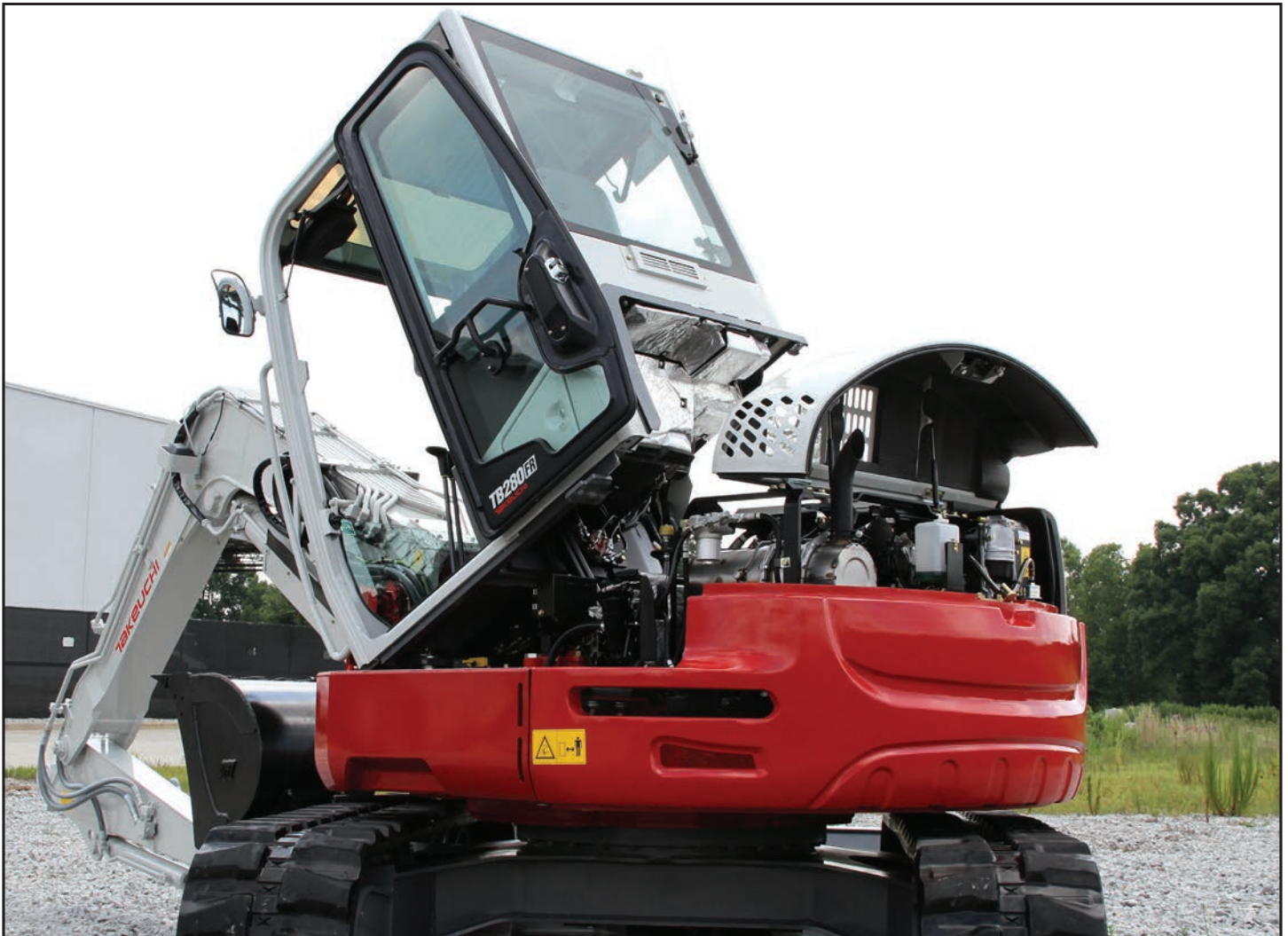
A tilt-able cabin and large lockable service hoods provide outstanding maintenance access.
