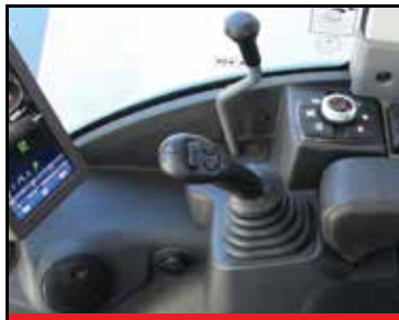
Hydraulic Pilot Controls
